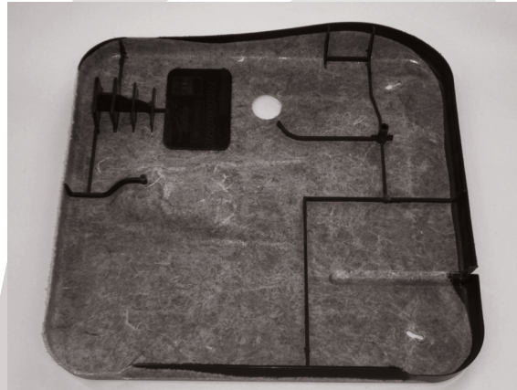
Picture 4: Three dimensional, structural very thin hybrid material mainly made from natural fibres with plastic reinforcement structure presented by Johnson Controls.
