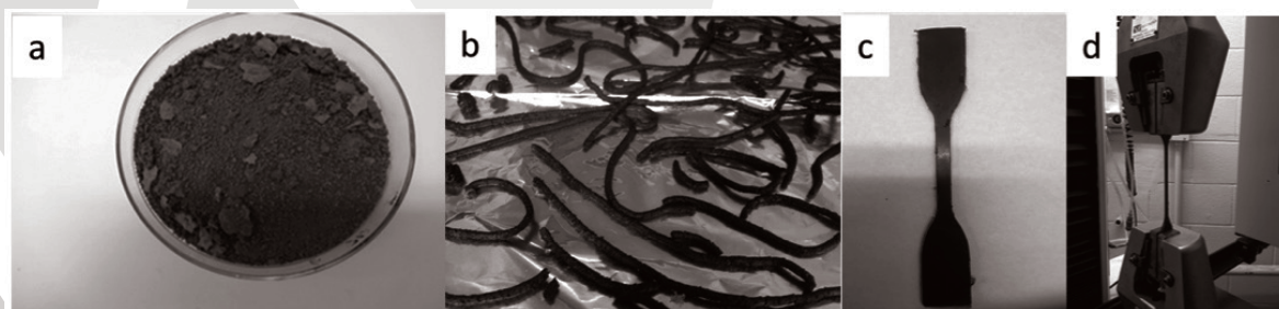
Figure 1: Residual microalgae biomass (a); Residual microalgae biomass plasticized with glycerol and urea (b); Green composites PBAT/RMB (80/20 wt) (c) and Green composites tested in Instron (d).
