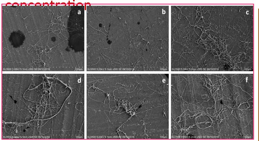
SEM images of electrospun nanofibers of SA with PEO with different concentrations of SA (a) 15 wt.%, (b) 12.5 wt.%, (c) 10wt.%, (d) 7.5 wt.%, (e) 5 wt.%, (f) 2.5 wt.% w.r.t. PEO
