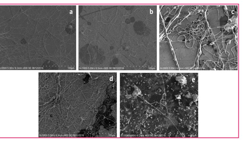
Scanning electron microscope (SEM) images of electrospun nanofibers of SA with PEO in presence of different solvents (a) Acetone, (b) Methanol, (c) Chlorofrom, (d) Ethanol, (e) Water
