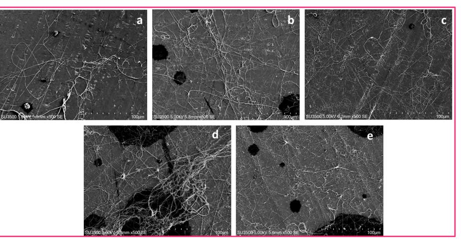
Scanning electron microscope (SEM) images of electrospun nanofibers of SA with PEO in different amount of ethanol (a) 1 mL, (b) 2 mL, (c) 3 mL, (d) 4 mL, (e) 5 mL.
